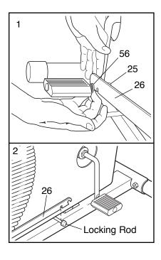
Clip the Link Arms (26) onto the lock rod as shown in drawing 2.
